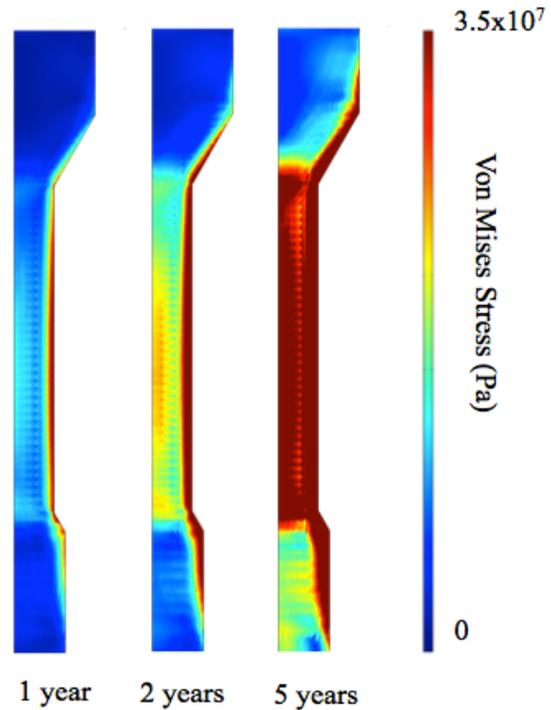
Figure 1: Central Reflector Von Mises Stress at Various Core Lifetimes
